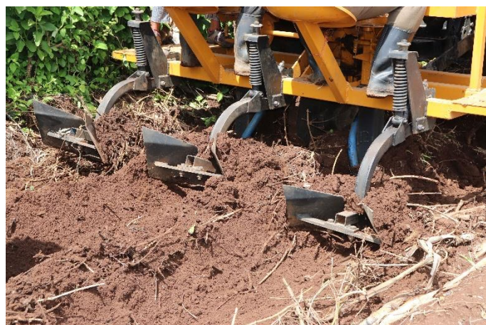
Figure 53 Demonstrating the use of rippers in land preparation
