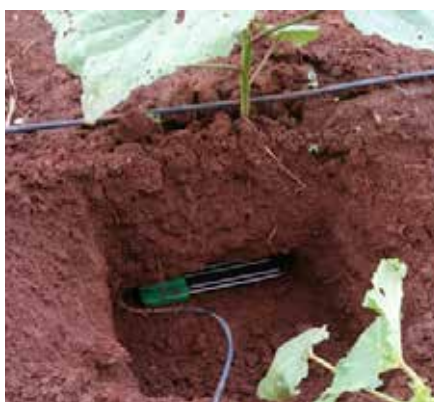
Figure 1: Soil moisture and temperature sensor installation at Sokoine University of Agriculture.
