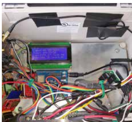
Figure 2: Wireless precision irrigation controller developed by University of Florida and SUA.
