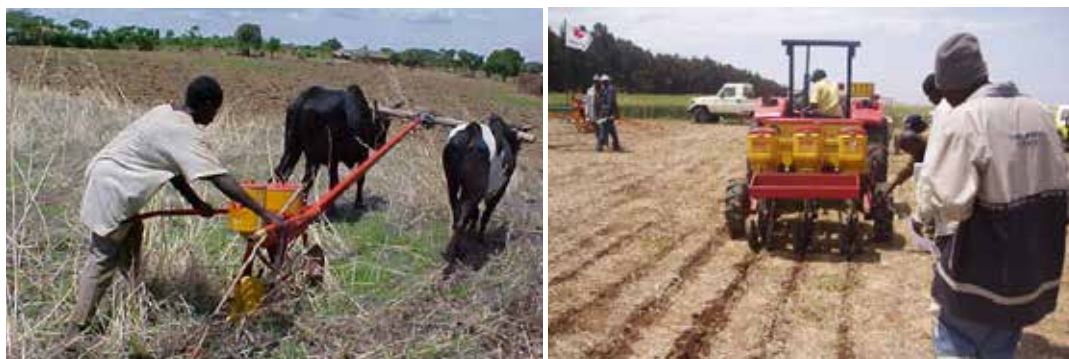
Plate 7: Animal drawn direct seeder (left) and tractor drawn seeder (right)
