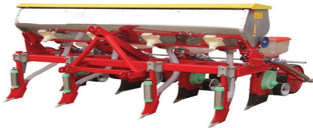
Figure 28. A tractor drawn sorghum planter. Source: Abo Al-kheer, 2010
