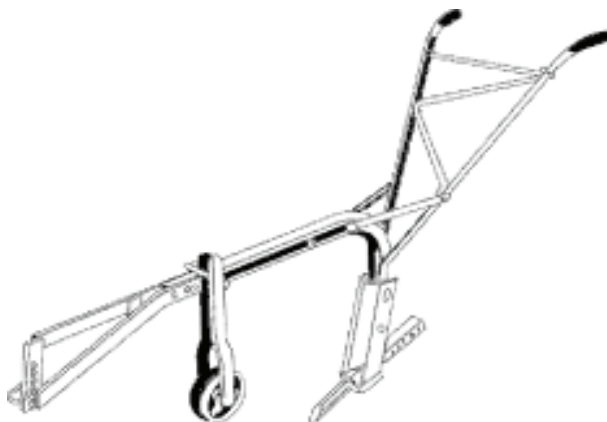
Figure 26. A sub-soiler (left) A sub-soiler fixed on oxen plough (right)
