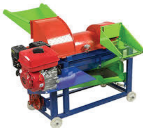
Figure 33. Motorized sorghum thresher. Source: https://www.cornmachine.com
