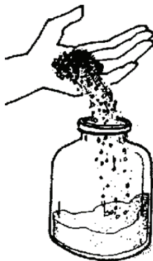
Figure 35. Salt moisture testing method
